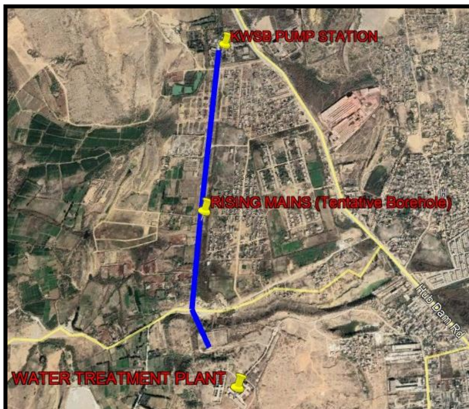
Figure 4: General Layout of the KWC, including the Pump Station and the Treatment Plant.
