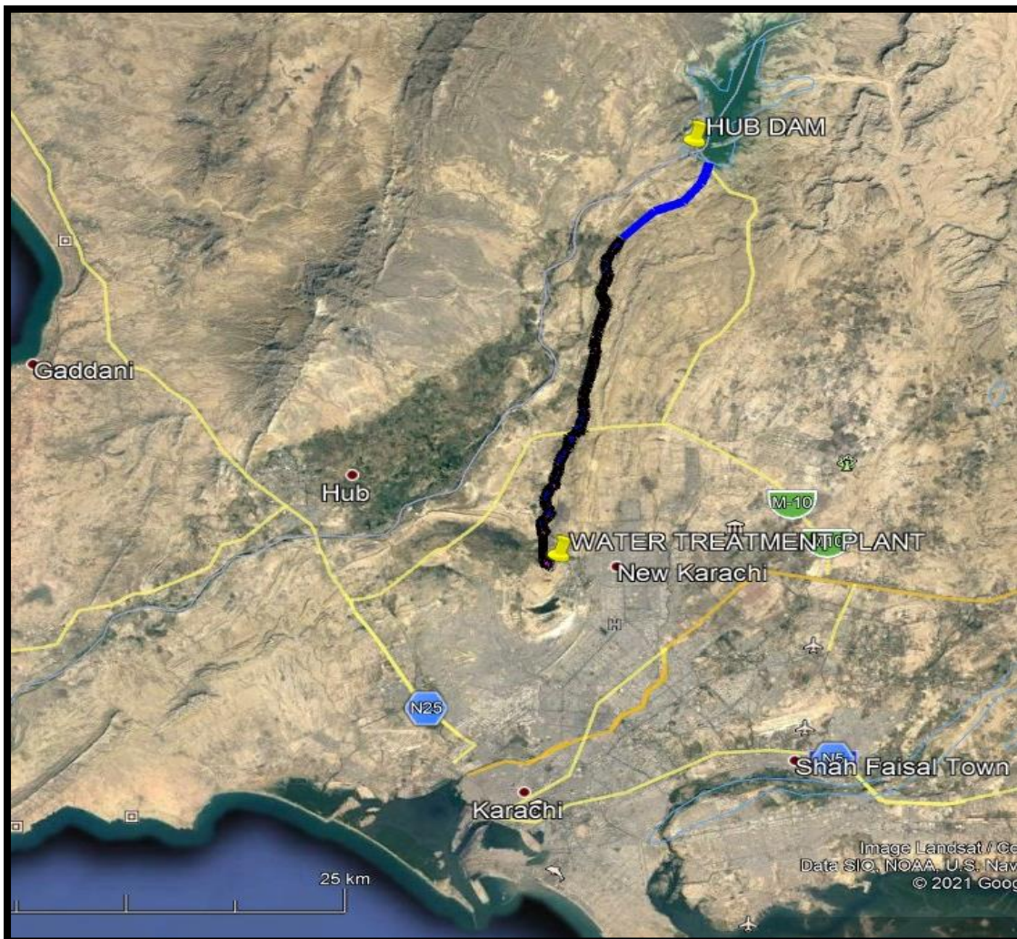
Figure 2: General layout of the KWC (in black) and the WAPDA Canal (in blue).
